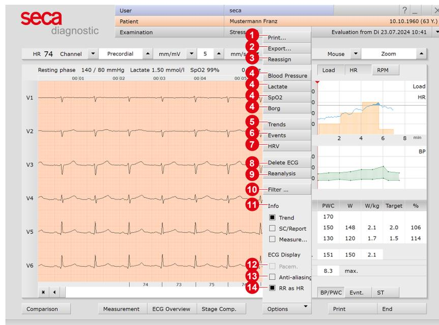
Fig. 42: Evaluation of stress ECG, Options menu
