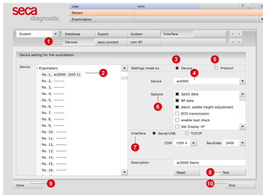
Fig. 12: Connecting training devices with seca diagnostic
