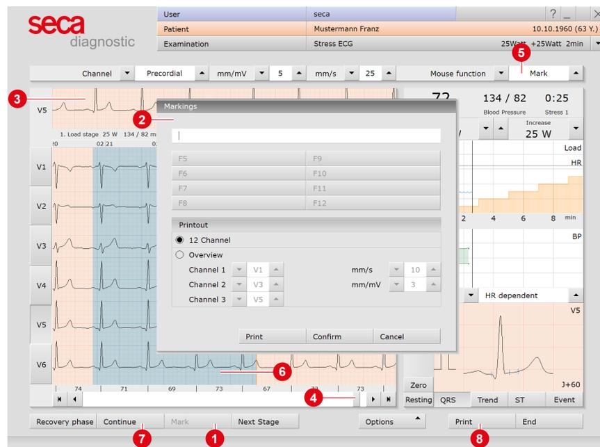
Fig. 28: Stress ECG recording, editing options
